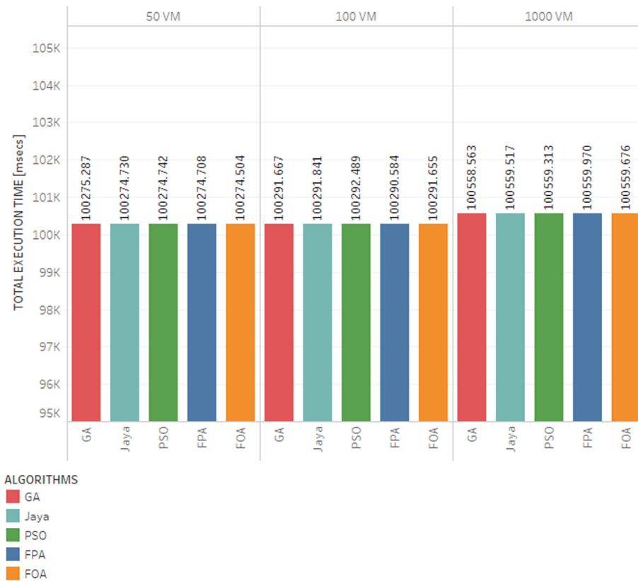
Fig. 12. Total execution time (ms) for 100,000 tasks and (a) 50VMs (b) 100VMs (c) 1000 VMs.
