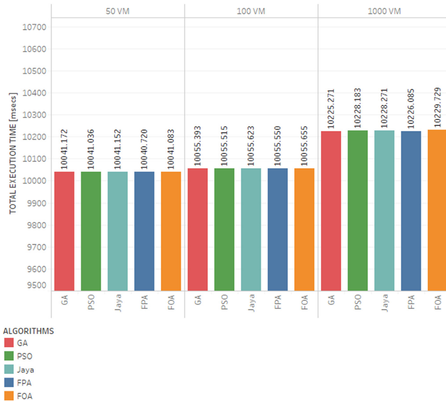
Fig. 11. Total execution time (ms) for 10,000 tasks and (a) 50VMs (b) 100VMs (c) 1000 VMs.
