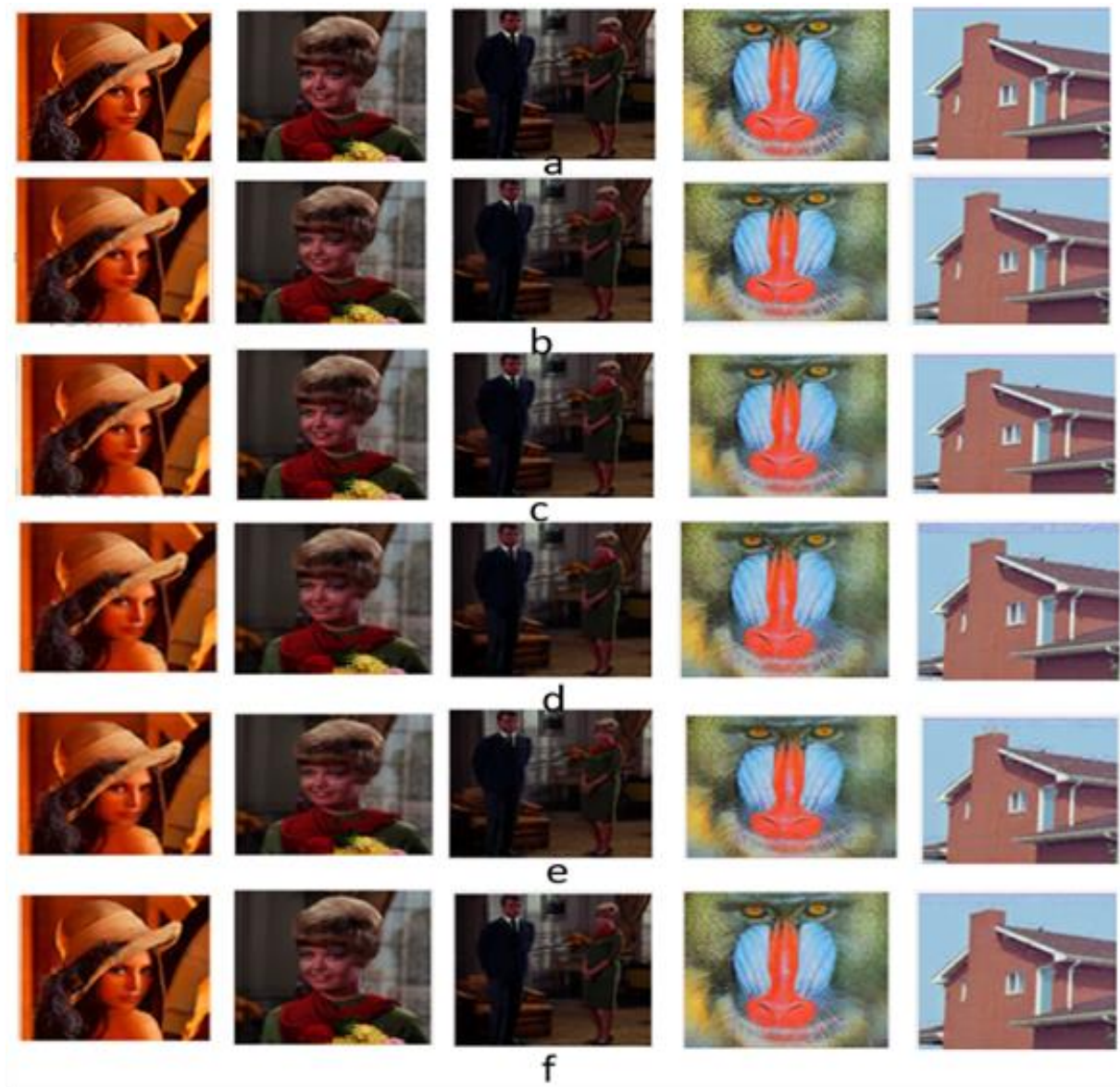
Figure 4. Reconstructed Lena, Zelda, Couple, Baboon and House image by using different ABCS methods (a) original image, (b) BCS-SPL, (c) STD-BCS-SPL, (d) ENT-ABCS, (e) EABCS, (f) FABC at 0.5 sampling rate.
